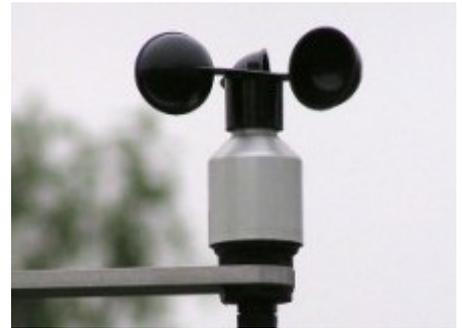
**The Challenge-** Your challenge is to design something that can measure the wind speed. Create an anemometer that features free spinning cups that spin faster as the wind increases. The wind should blow into the cups pushing them away. The faster the wind the more force it has to push the cups and the faster they spin. You can measure the wind strength by comparing how many times the anemometer spins around every 10 seconds.
